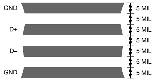
Figure 22. Typical Arrangement of Signal Tracks
